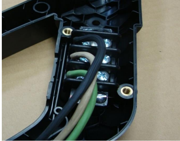
Fig.6-19 Terminal Block Wiring
