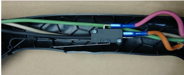
Fig. 6-17 Switch Wire Location
