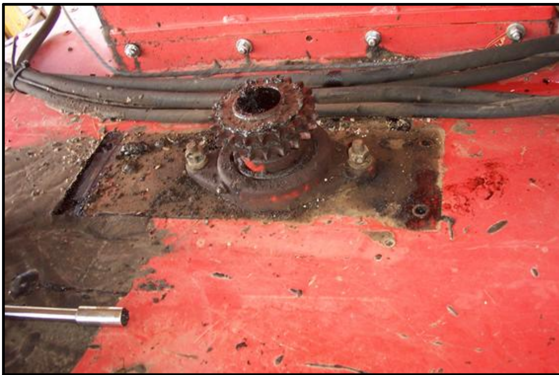
Fig. 6-5 Removal of Motor Mount Assembly
