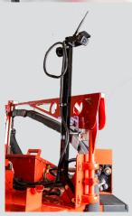
Telescoping mast and adjustable camera expands the field of vision.
